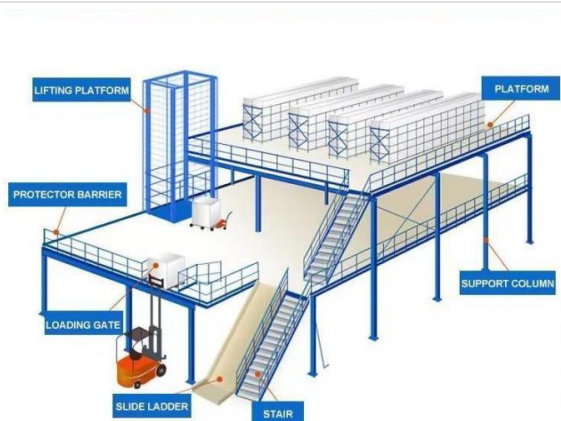
STAIRS AND HYDRAULIC LIFTING PLATFORMS The lifting platform is used to transport goods up and down between floors, with a large practical carrying capacity, smooth lifting and lowering, reducing manual handling, and slides can be configured according to needs.
