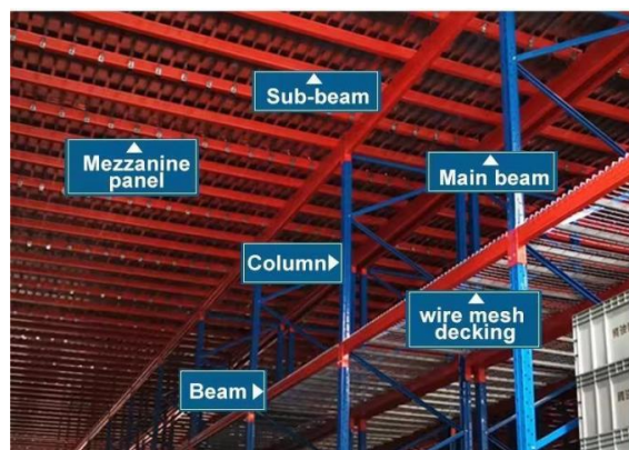
BEAM Complying with mechanical design, each position has been calculated and measured to ensure outstanding load-bearing capacity, safety and stability.
