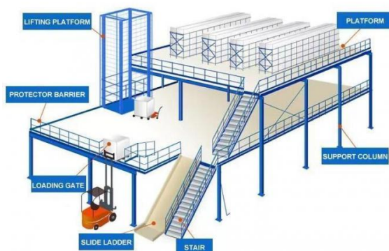
STAIRS AND HYDRAULIC LIFTING PLATFORMS The lifting platform is used to transport goods up and down between floors, with a large practical carrying capacity, smooth lifting and lowering, reducing manual handling, and slides can be configured according to needs.
