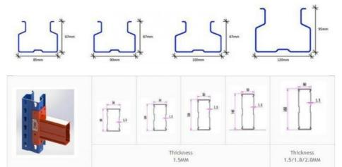
Beam consist of hollow profiles with beam end connectors welded to each end for connection to the uprights. Beam end connectors are available with 3 or 4 pins. The beams have electrostatic epoxy powder coating (standard finish orange RAL 2004). Safety pins can also be used to prevent the beam from unhooking.
