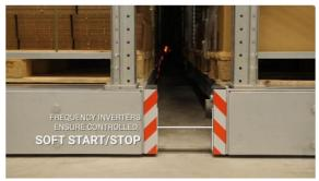
The electronically controlled MOVO high-load racking system runs on in-ground rails and can carry bay loads of up to 24 tons at racking heights of up to 15 meters. While state-of-the-art sensor technology and variable control options ensure ease of operation and absolute safety.
