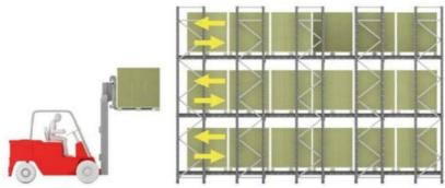
Drive through pallet racking (FIFO - First in, First out)
