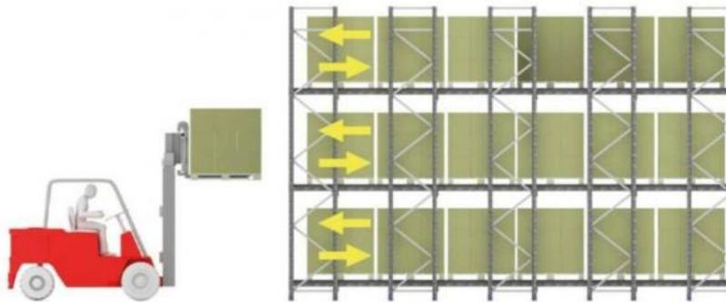
Drive through pallet racking (FIFO - First in, First out)
