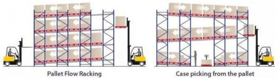
Fluent shelf working principle
