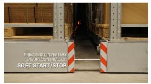
The electronically controlled MOVO high-load racking system runs on in-ground rails and can carry bay loads of up to 24 tons at racking heights of up to 15 meters. While state-of-the-art sensor technology and variable control options ensure ease of operation and absolute safety.
