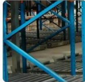
Inclined tie rod
