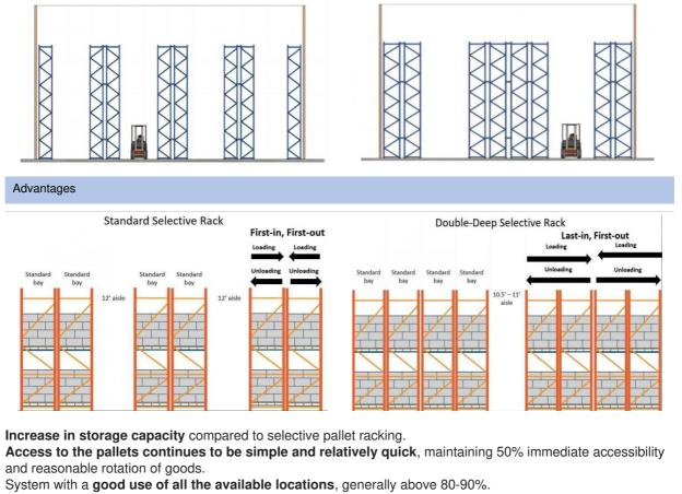
Intermediate system between an adjustable or selective racking system and a high-density compact system. LIFO (Last in, First out) system, where the last pallet deposited on the racking will be the first one to leave. More efficient system, which eliminates unnecessary aisles and increases the use of available space. Double deep pallet racking systems adapt to any type of unit load.
