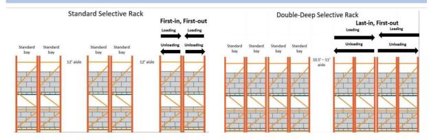
**Increase in storage capacity** compared to selective pallet racking.
