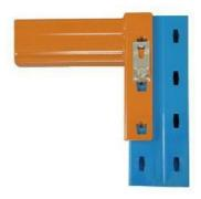
According to the beam section size, 3-hole or 4-hole hooks can be selected to meet different bearing capacity requirements. There is a safety lock at the connection to lock the beam. The safety lock is preinstalled at the factory, which improves the installation work efficiency and avoids the safety problem without a safety lock.
