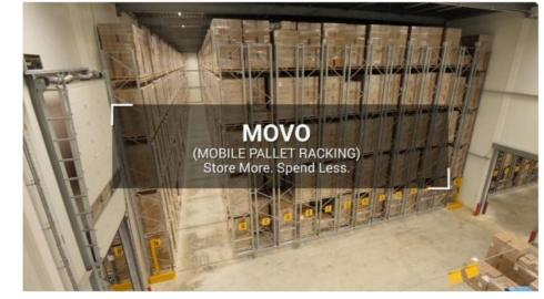
Trolley length: up to 90m Rack height: up to 15m
