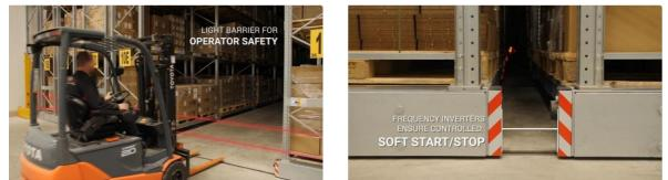
The electronically controlled MOVO high-load racking system runs on in-ground rails and can carry bay loads of up to 24 tons at racking heights of up to 15 meters. While state-of-the-art sensor technology and variable control options ensure ease of operation and absolute safety.
